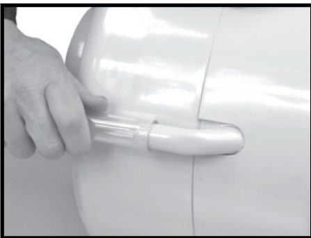
Step 7. Fit oil return tube and position tube to drain oil back to machine enclosure, sump or collection vessel.
