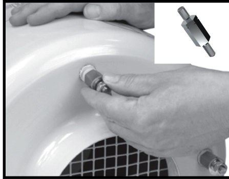
Step 2. Fit four case studs with the notched edge facing towards the Filtermist unit (supplied with unit).
