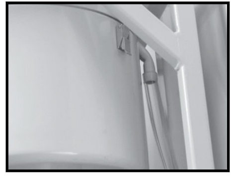
Step 6. Fit oil return tube and position tube to drain oil back to machine enclosure, sump or collection vessel.
