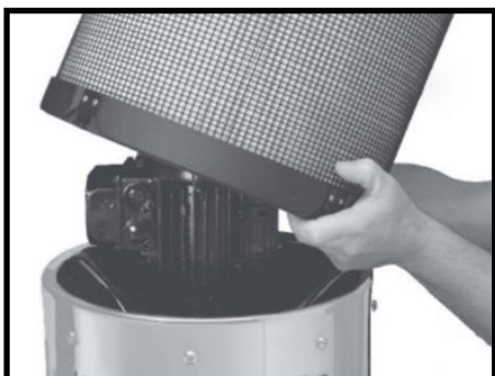
Step 4. Check the afterfilter (if fitted) and replace if necessary.
