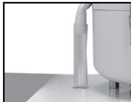
Step 3. Check the oil return hose for damage and blockage.
