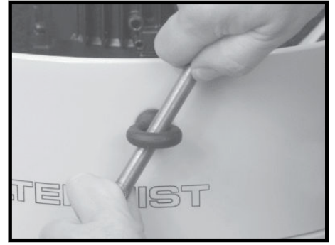
Step 3. Tighten eyebolts until horizontal.
