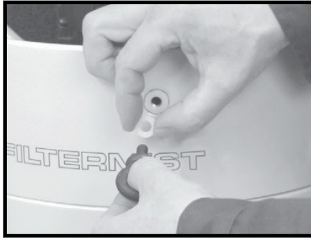
Step 2. Screw in four eyebolts with nylon washers.
